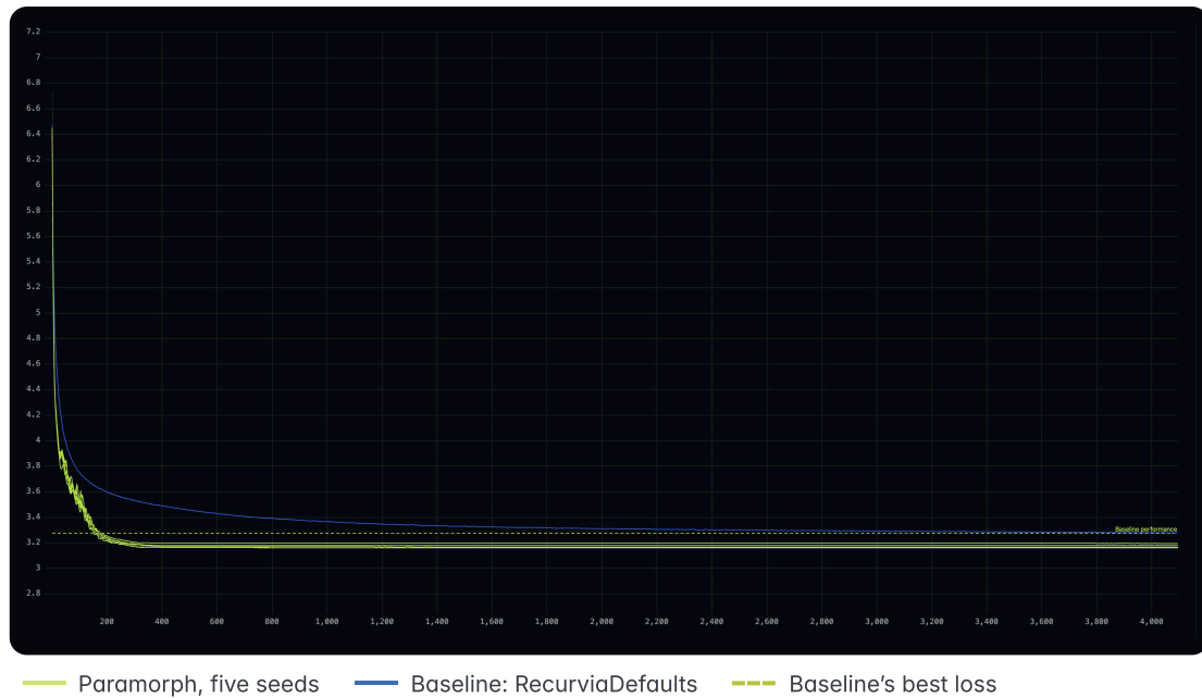
Figure 17. The 4,096-step budget. Paramorph reaches the baseline's best loss in under 200 steps and finishes about 3% lower in loss; the fixed baseline improves only slowly over the remaining budget. Horizontal axis: decision steps of 100 batches.
